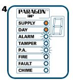
6) Turning Chime On and Off Panel must be in 'day' mode
