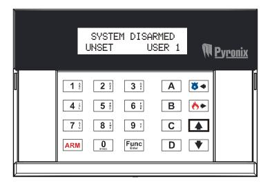
Similarly, if the down arrow key is pressed, the next most recent entry will be displayed. The up and down arrow keys may be used to scroll through the last 100 events in the event log. An error tone will be produced if an attempt is made to scroll outside either end of the event log.
