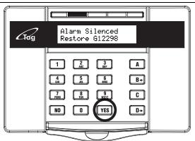
When the time is displayed, enter the number given to you by the ARC. 'Engineer Restore Performed' will be displayed once the correct number has been entered.
