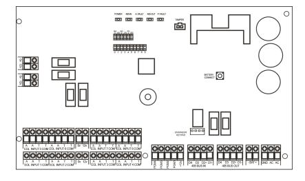
NOTE: The D2+ terminal must not be connected.
