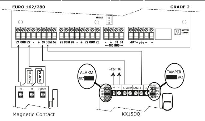
The above wiring example shows the connections for a Grade 2 KX15DQ PIR detector.
