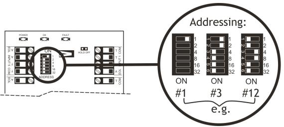
**NOTE**: The addressing is done by adding the relevant numbers on the dip switches:
