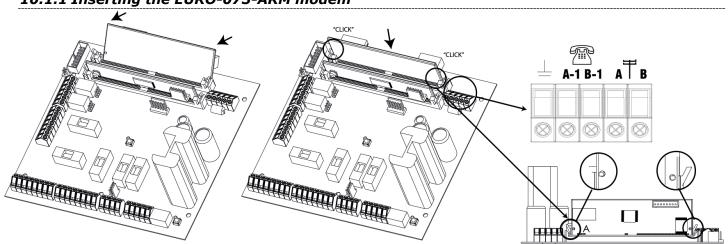
NOTE: Power down the EURO control panel before inserting the EURO-073-ARM modem
