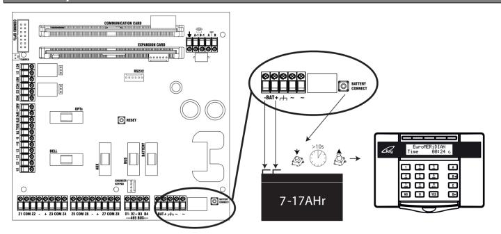
**NOTE:** The battery connect button is only used if no mains is present and a battery power up is required.
