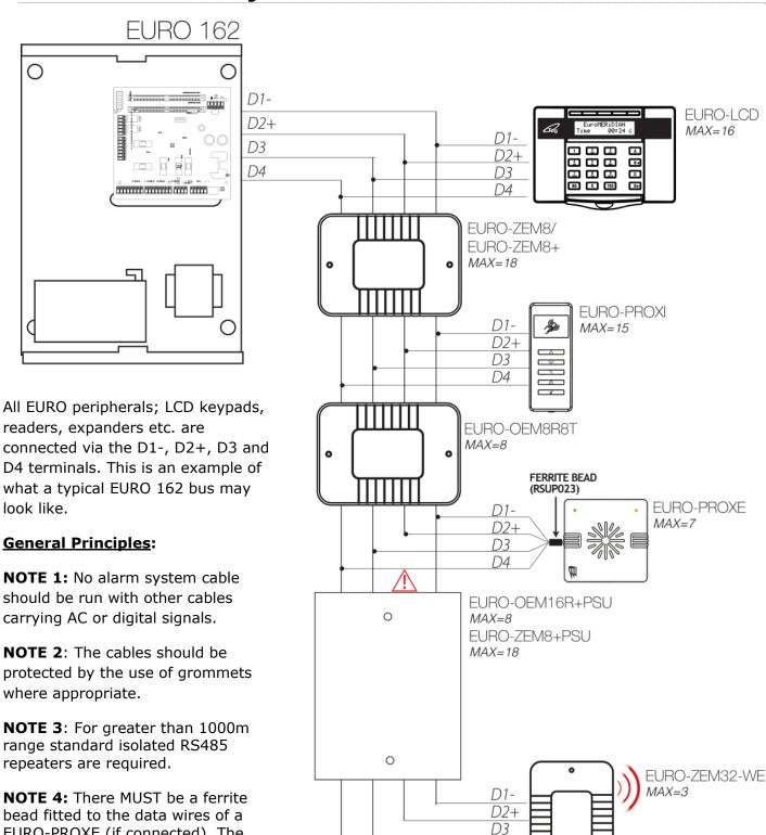
NOTE 5: (IMPORTANT!) If an expansion module with a power supply on board is connected, the D2+ terminal MUST NOT be connected between the main bus and module.
