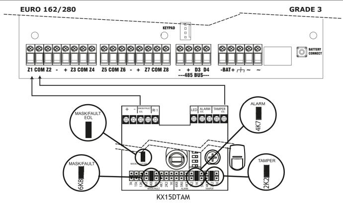
The above wiring example shows the connections for a Grade 3 KX15DTAM detector.
