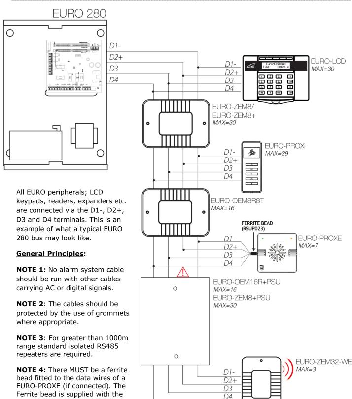
NOTE 5: (IMPORTANT!) If an expansion module with a power supply on board is connected, the D2+ terminal <u>MUST NOT</u> be connected between the main bus and module.
