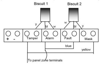
Please note that when using masking you must program the masking biscuit (iD 2 in the above example as 'fault') and then pair the corresponding inputs using the 'paired input' attribute. It is possible to spur off at this point to a further detector(s).
