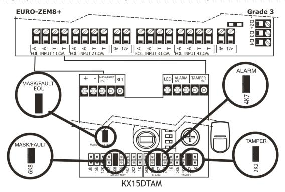
The above wiring example shows the connections for a Grade 3 KX15DTAM PIR.
