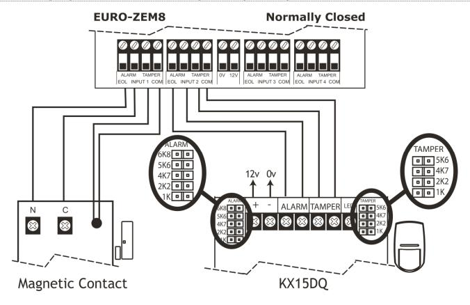
The above wiring example shows the normally closed connections for a KX15DQ PIR.
