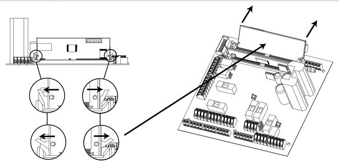
**NOTE:** Power down the EURO control panel before removing the EURO-073-ARM modem
