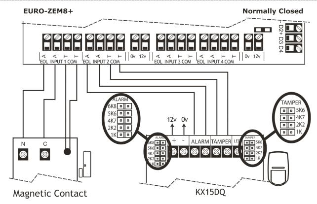
The above wiring example shows the normally closed connection for a KX15DQ PIR.
