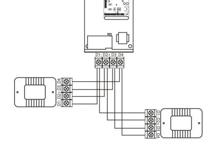
Daisy Chain Wiring Diagram
