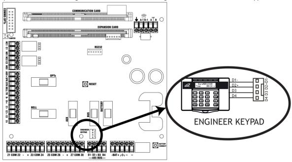
**NOTE:** Before an Engineer keypad is enabled, it should be addressed as an additional keypad on the EURO control panel before operation. See page: 26 for adding keypads to the EURO control panel.
