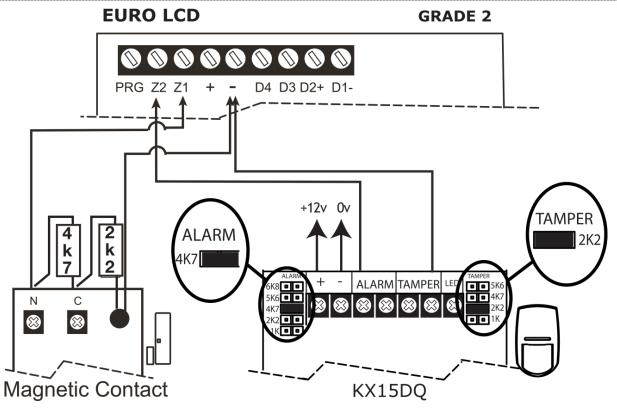
The above wiring example shows the connections for a Grade 2 KX15DQ PIR.
