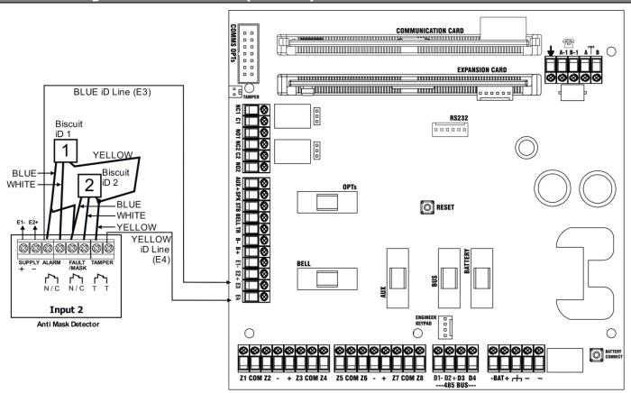
For separate fault and mask relays use the below configuration
