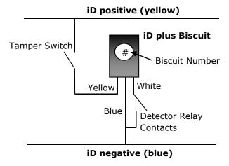
The third, WHITE, connection to the biscuit is used for the switch contact.
