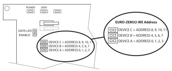
The EURO 162/280 will support both wired and wireless expanders on the same bus. Wireless sounders and Keyfobs must be learned to Address 0.
