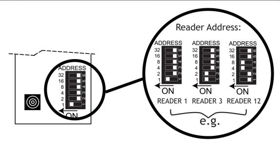
**NOTE**: The addressing is done by adding the relevant numbers on the dip switches:
