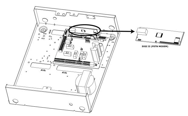
The EURO-073-ARM card is a 2400bps modem and enables communication via PSTN line using Fast Format or SMS as well as remote uploading/downloading. This works through the telephone terminals on the EURO 162/280. The connections are as follows:
