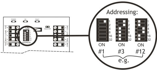
**NOTE**: The addressing is done by adding the relevant numbers on the dip switches: For example: Dip switch 1 and 2 are only ON = Address 3. Dip switch 1 and 16 are only ON = Address 17 etc.
