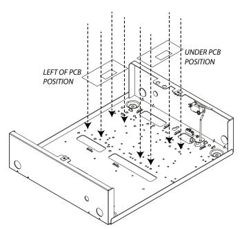
On the EURO 46 Large, the Digi-1200 (PSTN) modem can be installed underneath the EURO 46 PCB or to the left of it – however the GSM must always be mounted in the 'left of PCB' position. Connecting the modem in the EURO 46S
