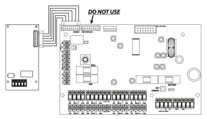
The DIGI-1200 (PSTN) modem enables communication via PSTN line using Fast Format or SMS as well as remote uploading/downloading.
