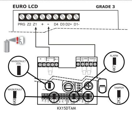
The above wiring example shows the connections for a Grade 3 KX15DTAM PIR.
