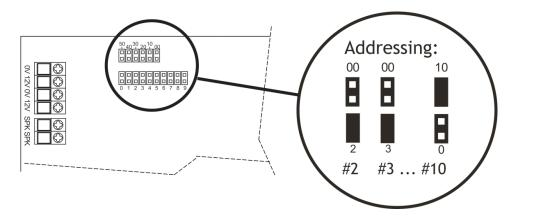
**NOTE**: The addressing is done by headers that represent the address. For example: If a header is placed on 00, and 9, the address is 9. If a header is placed on 20, and 3, the address is 23 etc.
