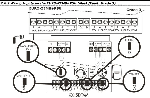
The above wiring example shows the connections for a Grade 3 KX15DTAM PIR.
