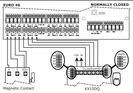
The above wiring example shows the normally closed connections for a KX15DQ PIR detector.
