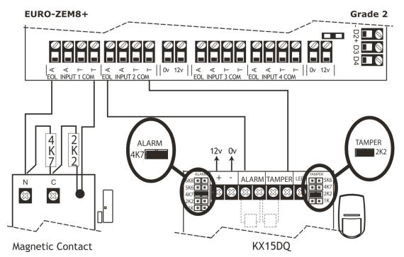
The above wiring example shows the connections for a Grade 2 KX15DQ PIR.
