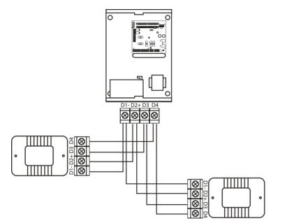
Daisy Chain Wiring Diagram
