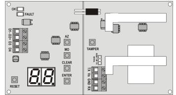
A total of 7 detectors can be programmed using the End of Line mode on a radio expander. The **`OK**' and **`FAULT**' LEDs relate to the RS485 connection to the EURO system.
