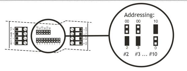
**NOTE**: The addressing is done by headers that represent the address. For example: If a header is placed on 00, and 9, the address is 9. If a header is placed on 20, and 3, the address is 23 etc.
