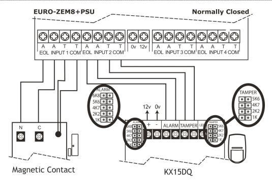
The above wiring example shows the normally closed connections for a KX15DQ PIR.
