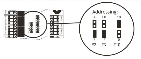
**NOTE**: The addressing is done by headers that represent the address. For example: If a header is placed on 00, and 9, the address is 9. If a header is placed on 20, and 3, the address is 23 etc.
