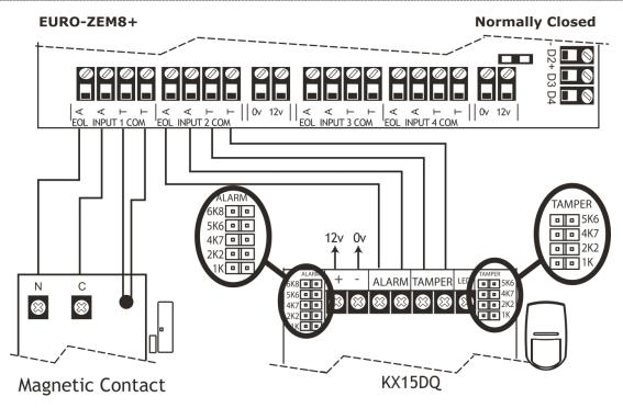
The above wiring example shows the normally closed connection for a KX15DQ PIR.
