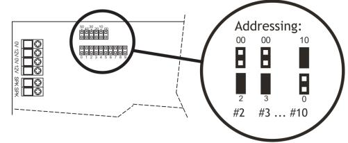
**NOTE**: The addressing is done by headers that represent the address. For example: If a header is placed on 00, and 9, the address is 9.
