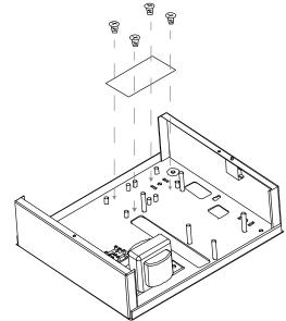
On the EURO 46 Small, the Digi-1200 (PSTN) or GSM modem should be installed to the left of the EURO 46 PCB.
