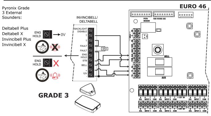
6.2 Grade 2 External Sounder Wiring with a Grade 3 Bell
