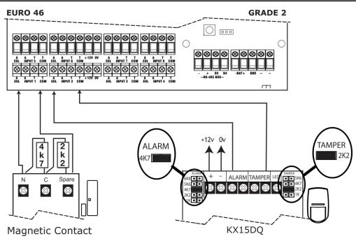
The above wiring example shows the connections for a Grade 2 KX15DQ PIR detector.
