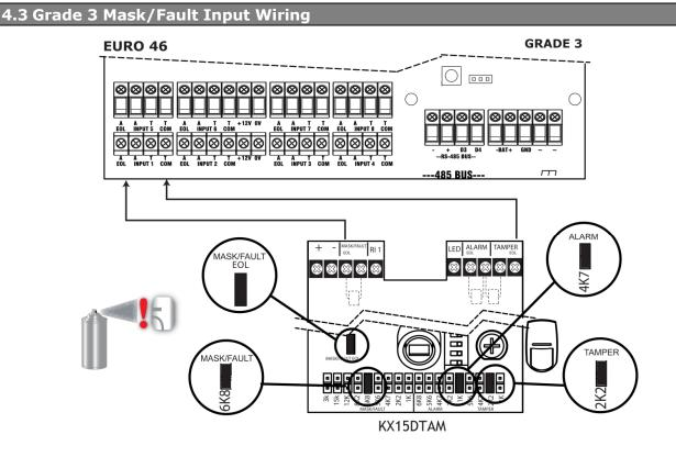
The above wiring example shows the connections for a Grade 3 KX15DTAM detector.
