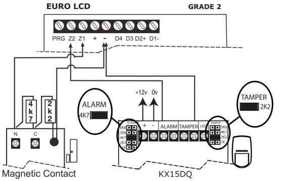
The above wiring example shows the connections for a Grade 2 KX15DQ PIR.
