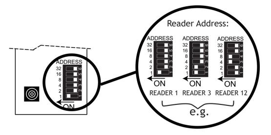
**NOTE**: The addressing is done by adding the relevant numbers on the dip switches: For example: Dip switch 1 and 2 are only ON = Address 3. Dip switch 1 and 16 are only ON = Address 17 etc.
