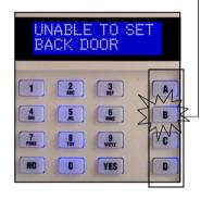
An appropriate **A B C D** key will flash to indicate within which area the fault exists.
