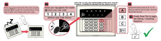
Controlling Outputs (switching gates, sprinklers, lights etc. if enabled by installer)
