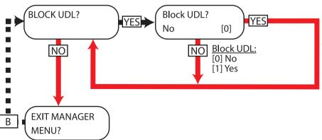
If enabled, this function will block any attempt made to dial into the control panel to upload and download information.
