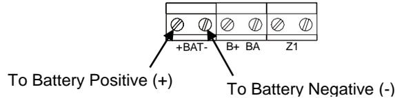
In order for the Atlas 4 to operate if the mains power is cut a battery back-up is required. Refer to 9.6 for battery specifications. Connect the battery to the terminals marked +BAT- on the PCB.
