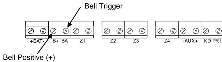
The bell Negative (-) should be returned to the BAT (-) connection on the PCB. The bell tamper must be connected to a tamper zone or connected as end of line zone. Bell box strobe connections should be linked together at the bell box.
