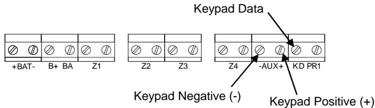
If more than one keypad is to be used, additional keypads can be wired in either daisy chain or star configuration. The RKP tamper must be connected to a tamper zone or connected as end of line zone.
