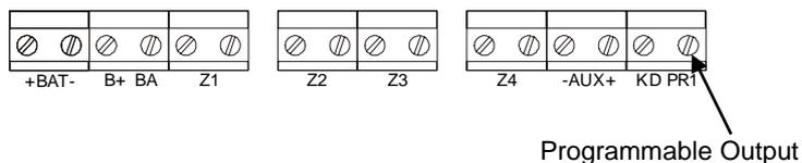
The Programmable Output is switched negative (-) on activation.
