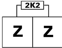
Wiring two or more sensors with end of line resistors to a single zone.
