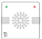
To arm/disarm the system using the external tag reader, present a pre-programmed tag to the centre of the device.
